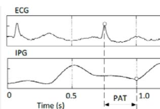
**Pulse arrival time measured using the footpad electrodes in a bathroom scale**
